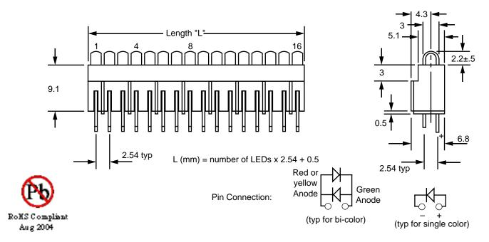
Specify part desired as follows: (XX = total number of LEDs in array, up to 16 maximum.)
