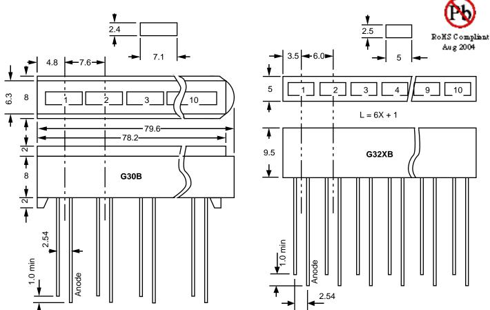
Specify part desired as follows: (X = total number of LEDs in array, 10 only for G30XB and up to 10 for G32XB.) G30B(or G32XB)/Order Code LED1 + Order Code LED 2 + ... + Order Code LED X For example: "G3210B/4I+4Y+2G" designates an assembly with 4 red, 4 yellow, and 2 green LEDs in that order.
