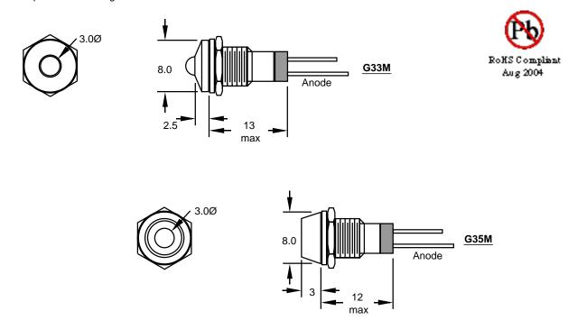
Specify part desired as follows: (X = total number of LEDs in array, and may be up to 8 maximum.) G33M/Order Code or G35M/Order Code
