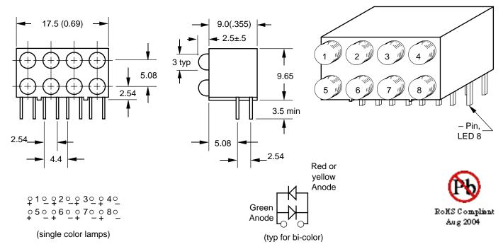
Specify part desired as follows:J784B/Order Code LED1 + Order Code LED 2 + ... + Order Code LED 8For example: "J784B/4H+4G" designates an assembly with 4 red LEDs on top and 4 green LEDs on the bottom. "J784B/(4H+4G)-RL" designates the same assembly with all lamps having reversed polarity.
